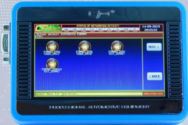
Last SYSTEM option gives you the possibility to format internal and external device memory.
