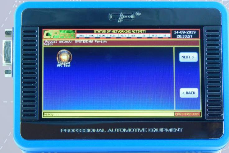
To update the device firmware place SD card in the SD card socket and start the update procedure using Upd Sys DBF From SD option.
