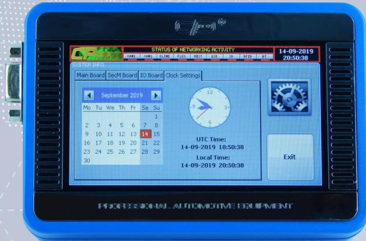
Clock Settings defines the device date and time in UTC format. Each of our devices has it's own datetime which is required for a proper system operation.
