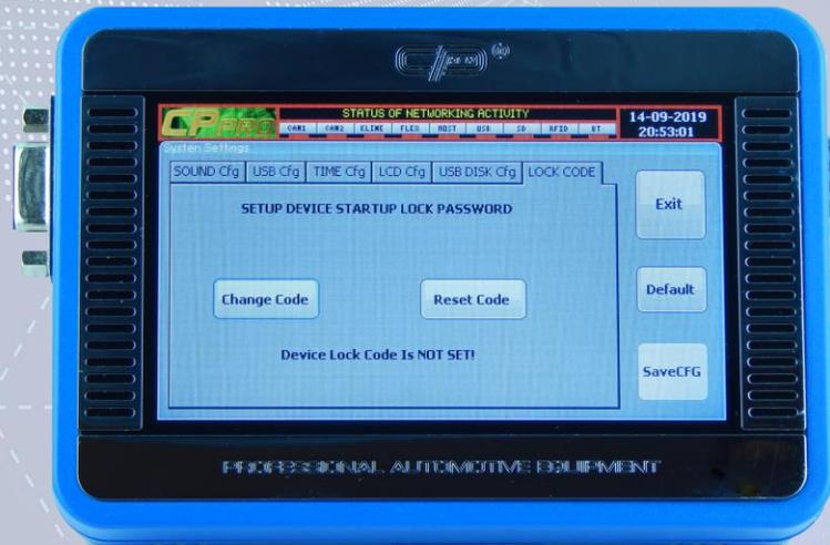
**LOCK CODE** If you would like to protect your device by the power on LOCK Password use option and provide your custom lock code.
