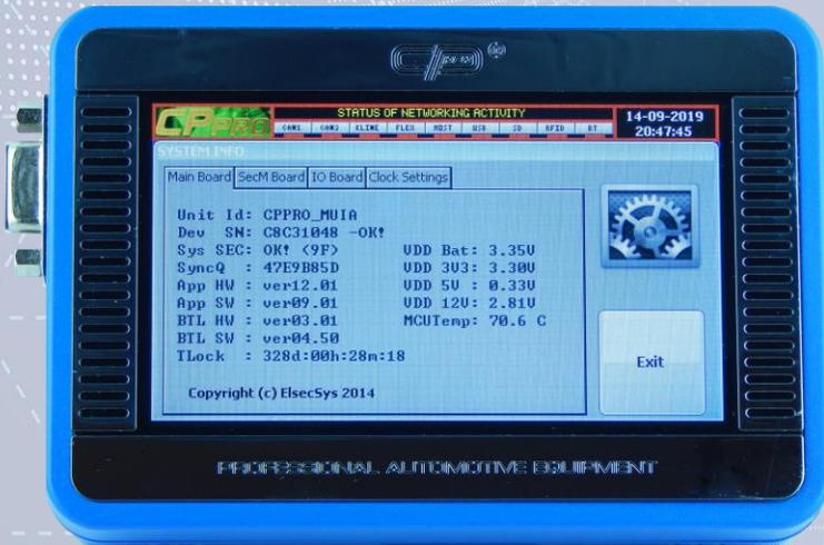
**Main Board** - section presents all of the most important details of CPPro device. You can find here information about the software versions, voltage details, current device temperature and TLock.
